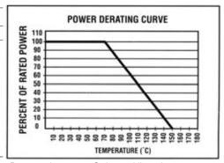
Power rating at 70° C derated linearly to 0% power at 150°C ( $P=E^{2}R$ ).
