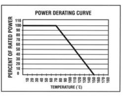
\_ Power rating at 70°C derated linearly to 0% power at 150°C ( $P=E^2/R$ )
