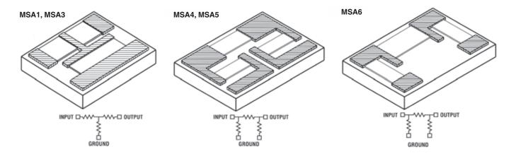
Wire and ribbon bondable and Flipchip thick film chip attenuators, printed and fired on 96% alumina. Provides attenuation accuracy for frequencies through 10 Ghz. Double layer terminations provide additional bonding surface. Abrasive trimming ensures optimum resistor stability. Diamond sawed for dimensional uniformity and accuracy. Advanced processing techniques, and Hi-Rel construction assure optimum performance.
