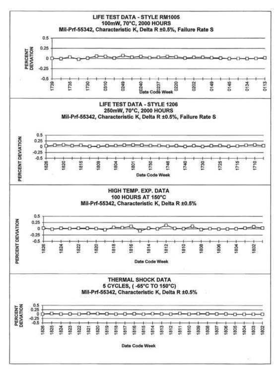
Back page of a Certificate of Conformance, containing data on Thick Film resistor products.
