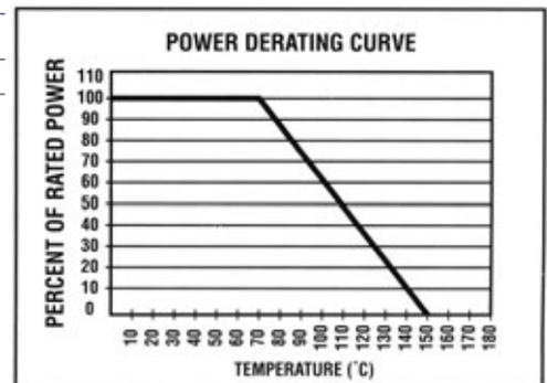
Power rating at 70° C derated linearly to 0% power at 150°C (P=E<sup>2</sup>/R).
