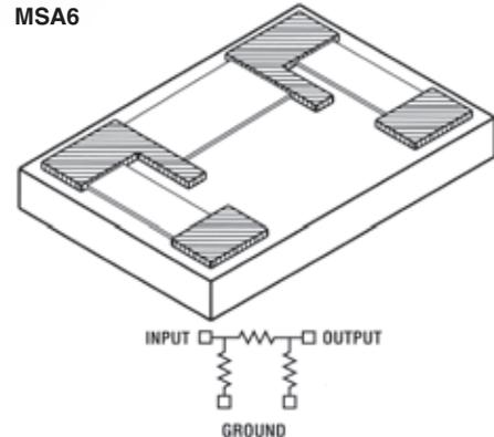
Wire and ribbon bondable and Flipchip thick film chip attenuators, printed and fired on 96% alumina. Provides attenuation accuracy for frequencies through 10 GHz. Double layer terminations provide additional bonding surface. Abrasive trimming ensures optimum resistor stability. Diamond sawed for dimensional uniformity and accuracy. Advanced processing techniques, and Hi-Rel construction assure optimum performance.
